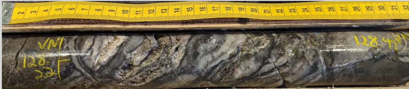
NQ sized drill core - Multiphase banded vein from hole 2XF-21-0015, depth 128.22 meters
